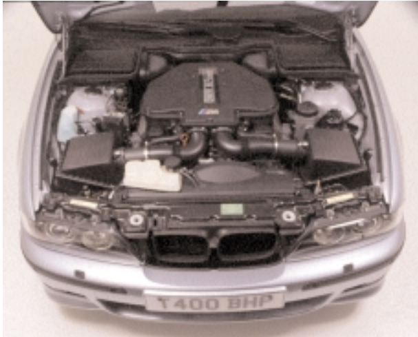
This is what lives underneath the sober-suited exterior. Motorsport's 5-litre V8 puts out 400 bhp and 369 lb.ft.
